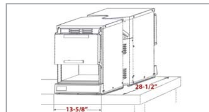
Two units fit back-to-back on a 28 1/2" (724 mm) shelf in a 13 3/8" (346 mm) space
